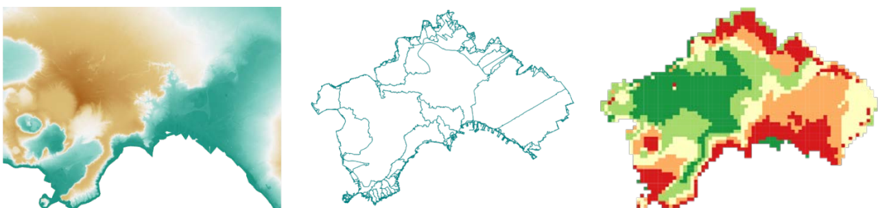
Figure 26: Naples area showing (left) runoff coefficient, and (right) its classification of imperviousness on a scale (1-5).
