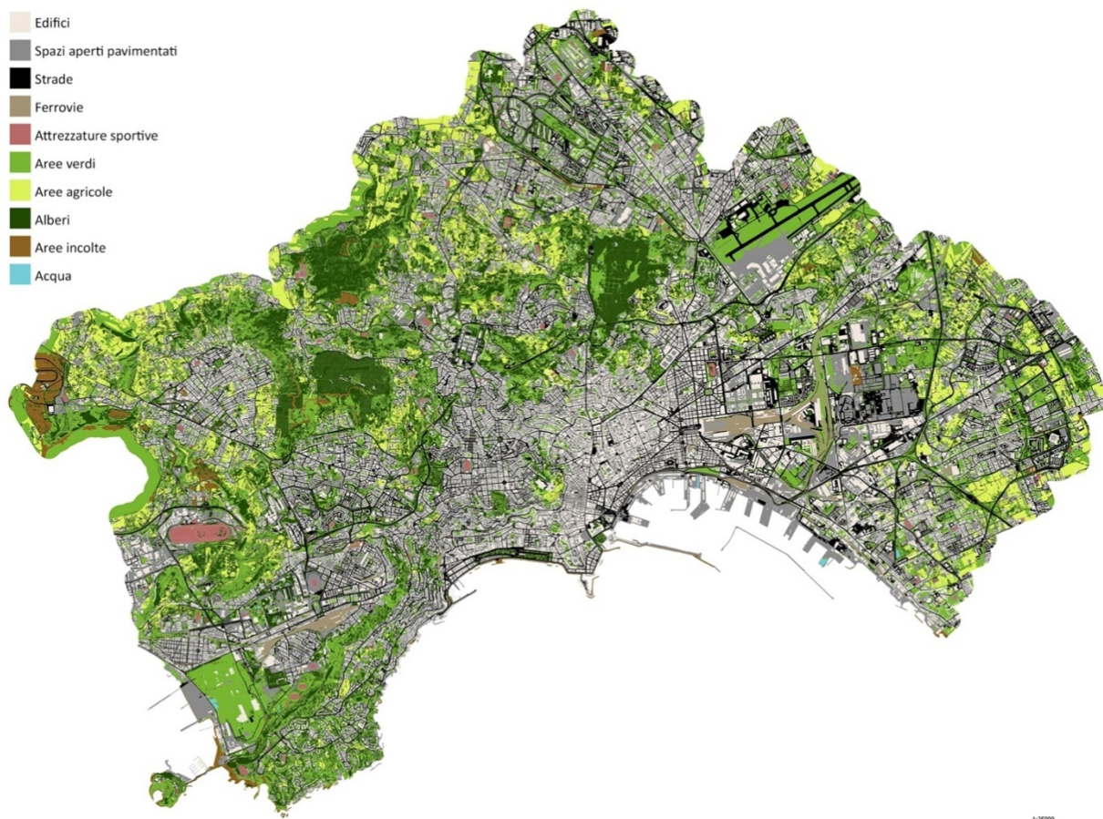
Figure 16: Reworked land use map used by simulation models of the “local effect” for heat waves and floods (Source: Municipality of Naples / PLINIVS-LUPT, CLARITY).
