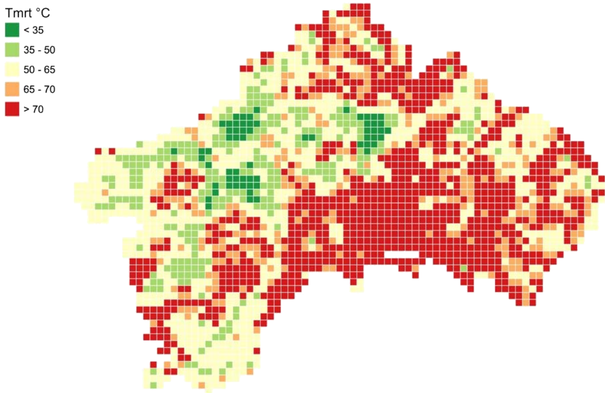
Figure 20: Mean Radiant Temperature map for a typical day of heat wave with air temperature of 41 °C (on grid 250x250m). (Source: PLINIVS-LUPT, CLARITY).
