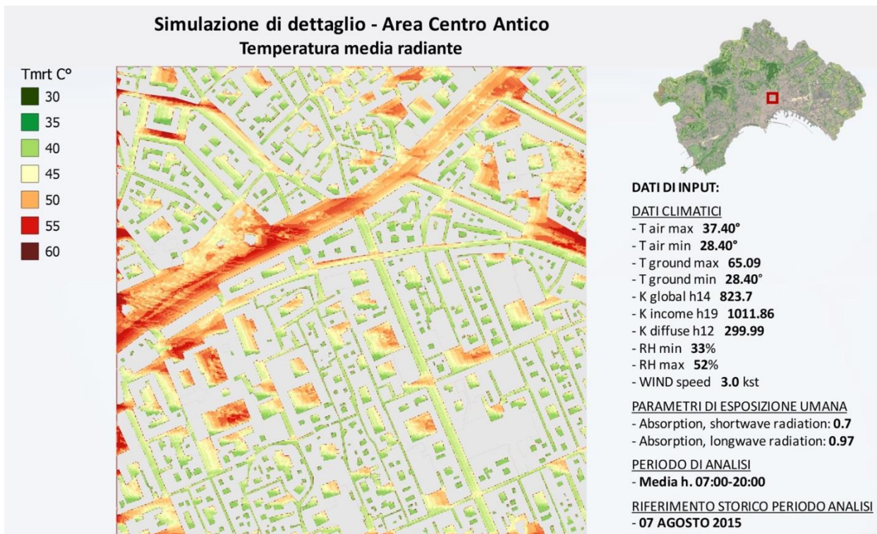
Figure 55: Detailed analysis of Tmrt in an area of the ancient centre, for a typical heat wave day with an air temperature of 36-37 °C. (Source: PLINIVS-LUPT, CLARITY project).
