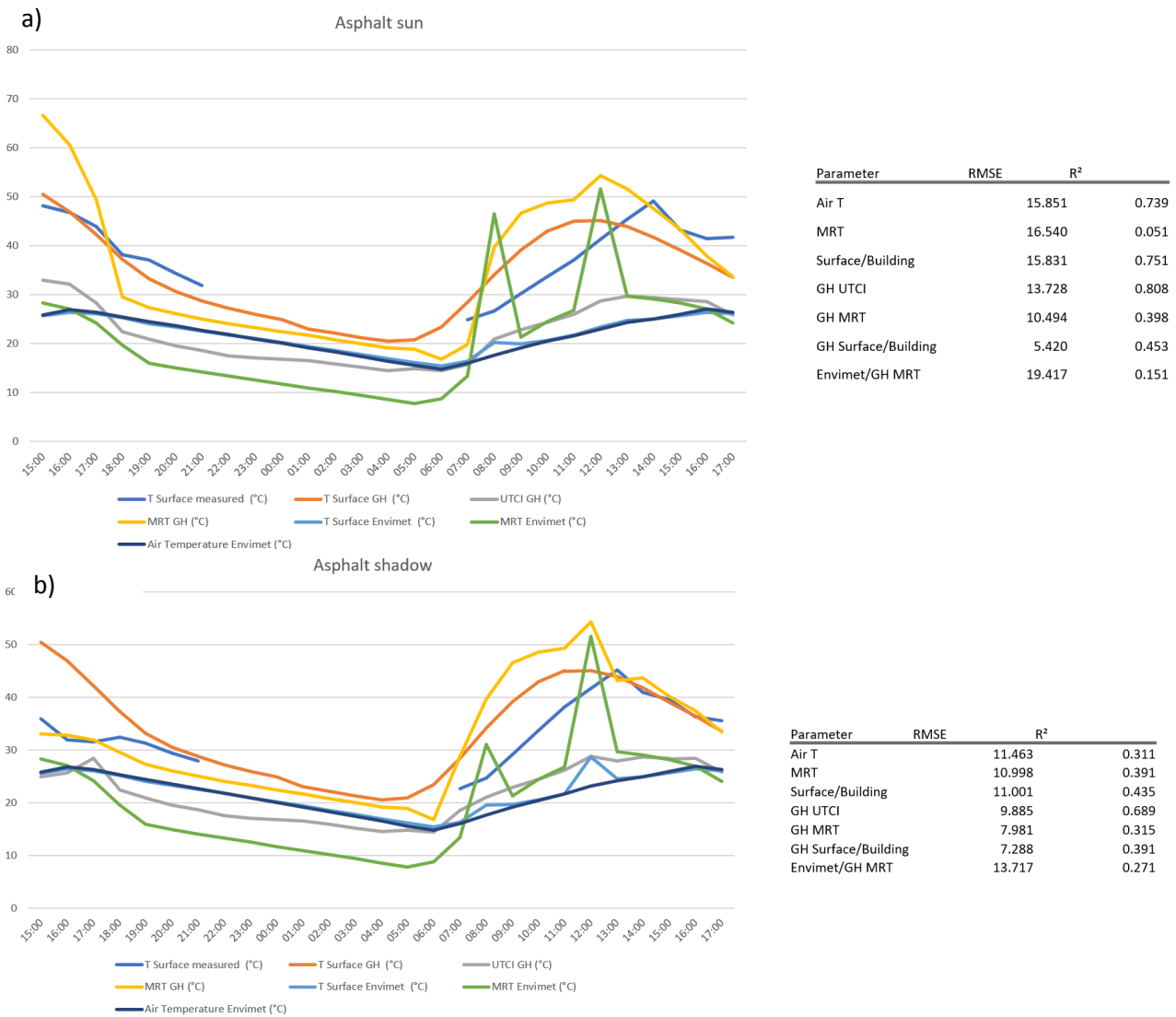
Figure 80: Comparison of measured and simulated values for the locations a) “asphalt sun” and b) “asphalt shadow”. The dark blue line represents the measured surface temperature, while the other lines represent values calculated either from ENVI-MET or Rhino/Grasshopper (GH).
